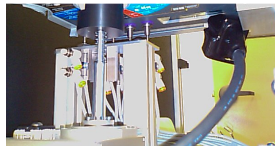
Stepper motor actuates knob and verifies the correct behaviour of the software.
