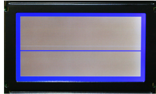
This LCD showed an errant row of pixels after a screen clearing command when the device went into standby.
